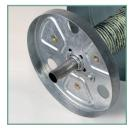
9-1/2" diameter drums allow for lower headroom requirements. An enclosed barrel houses the dead axle assembly and protects the factory lubricated springs from direct contact with environmental elements. The inherent strength provided by the spiral barrel minimizes axle deflection, providing smoother operation. Because the curtain is attached by screws and not seamed to the barrel, replacement of either independent assembly is cost-effective, quick and easy.
